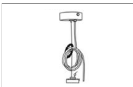
CEILING BASE TRANSPARENT CABLE ADJUSTABLE CABLE 3M, 5M or 7M MOUNTING GRIP
