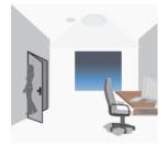
The light dims to stand-by period after hold-time and stays on selected minimum dimming level.
