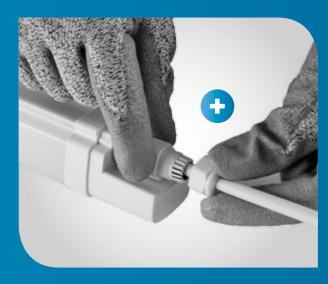
Complete the process by tightening the gland.
