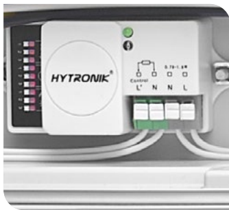
The application of a microwave motion sensor (RCR) helps provide light where and when it is necessary, which results in energy savings.
